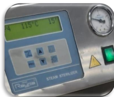
Figure 4. Sterilization process 15 minutes at 115 degrees C, 1.2 atm
