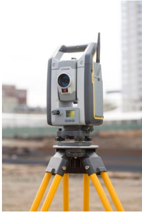
Figure 3. Total Station Trimble S7
