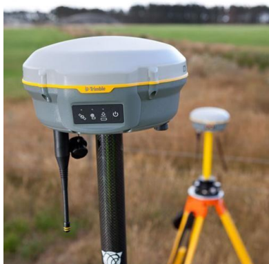
Figure 1. Receiver Trimble R8s
