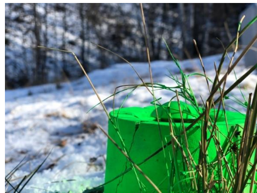
Figure 2. Ground Control Points (GCP)
