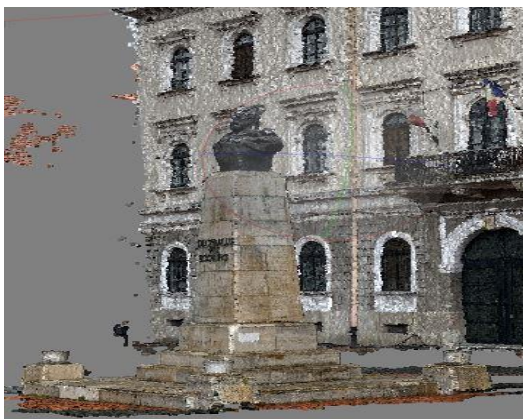
Figure 10. The result obtained from processing the photo using the Agisoft PhotoScan software
