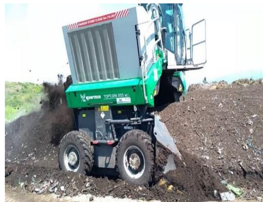
Figure 2. Compost tuner aerating compost piles
