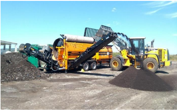
Figure 3. Compost screening with rotating drum
