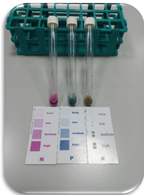
Figure 4. Vermicompost extract results for N, P, K
