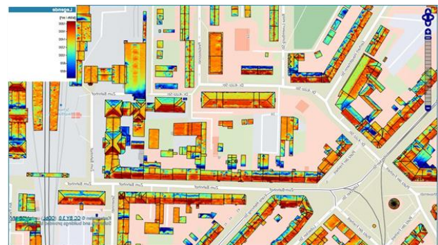
Figure 2. Solar radiation potential map for the city of Schwerin from Germany (source: http://solar.geocontent.de/schwerin/ )
