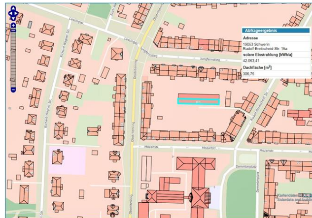
Figure 1. Solar potential map for the city of Schwerin from Germany – Data about address and annual solar radiation per surface (source: http://solar.geocontent.de/schwerin/ )
