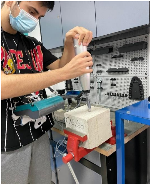
Figure 1. Test using sclerometer
