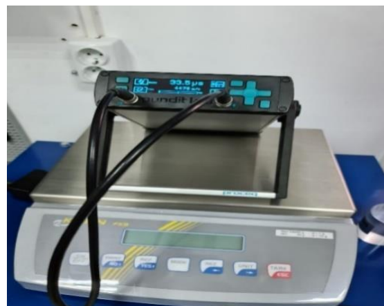
Figure 3. Electronic propagation speed measuring device
