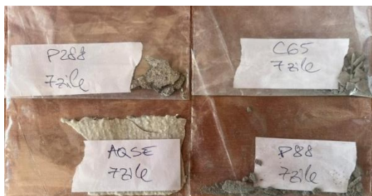
Figure 1. Pictures of waterproof mortars on day 7 after preparation.
