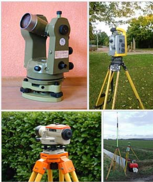
Figure 1. Surveying equipment: optical theodolite, robotical total station, optical level, RTK GPS base station
