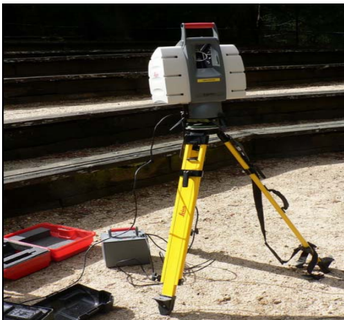
Figure 2. Lidar scanner that can be used for creating 3D models for buildings
