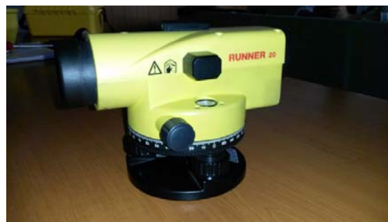
Figure 2. Leica grade level RUNNER 20
