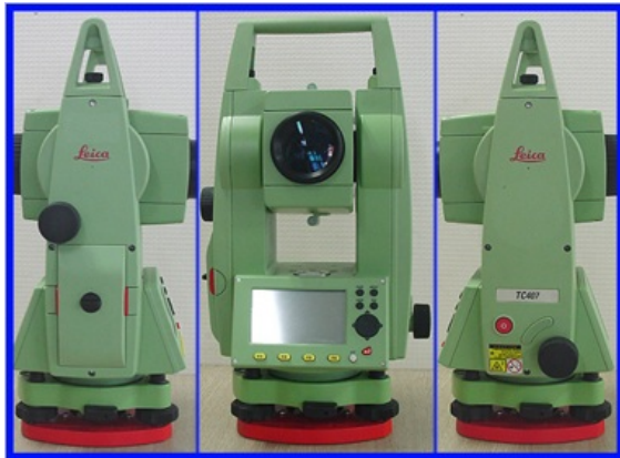
Figure 4. Leica TC407 total station
