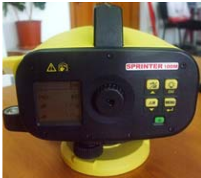
Figures 6, 7. Leica Sprinter 100M digital level
