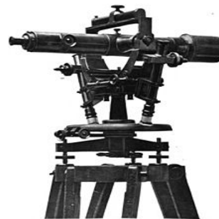
Figure 1. Eight-inch theodolite, c. 1898
