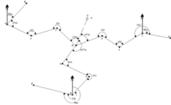
Figure 4. Graphical representation: traverse with hub point
