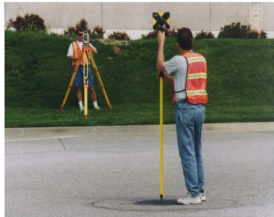
Figure 8. The measurement principle with reflector
