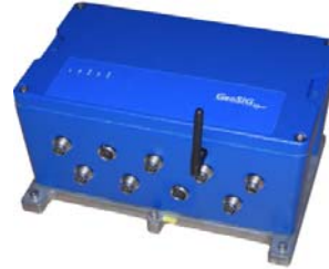
Figure 3. Digital Accelerograph GMS-18 GeoSIG.
