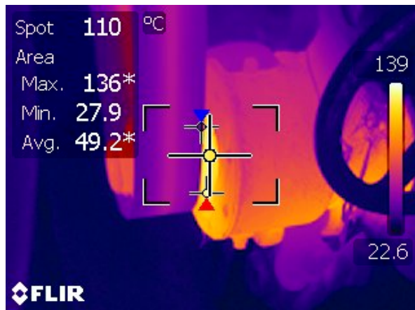
Figure 1. Sliding bearing overheated at 139°C
