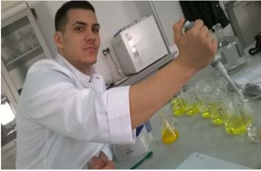
Figure 10. Determining the chlorine using the titrimetric evaluation
