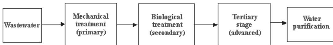
Figure 2. General scheme of all wastewater treatment plants
