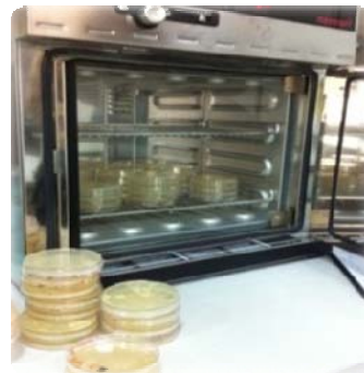
Figure 1. Thermostat for incubating samples (Microbiology lab CO3 – FIFIM)
