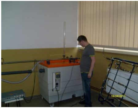
Figure 1 Experimental research on water hammer. Technical details of Armfield C7 Pipe Surg Apparature. Water supply stand Armfiel F1-10
