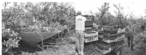
Figure 5. Umbrella harvester with shaker
