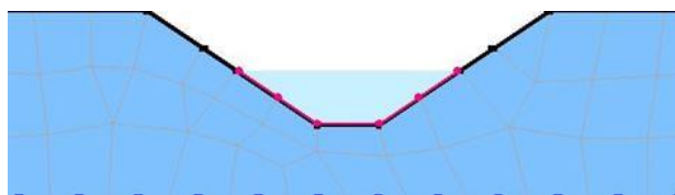
Figure 8. Hydraulic equal load lines
