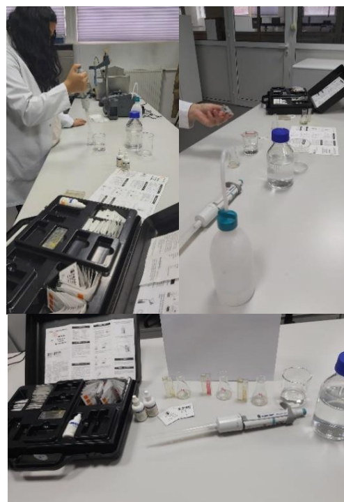
Figure 2. Ammonia test, nitrite test and nitrate test
