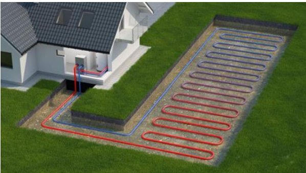
Figure 5. Heating pump water-soil
