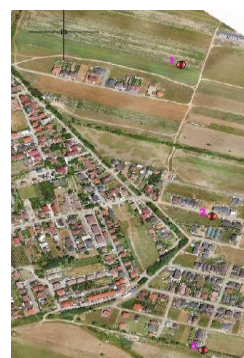
Figure 7. Marking control points on the ground
