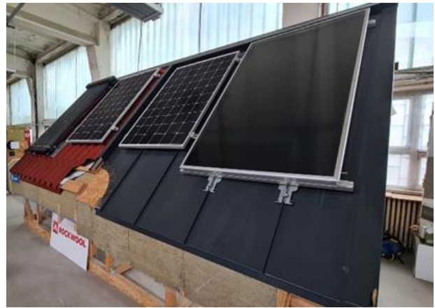
Figure 7. Different types of solar panels (Photo source: INCND URBAN-INCERC)
