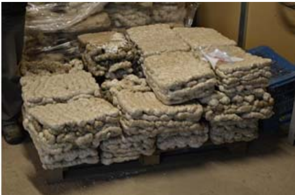
Figure 11. Pile with foam of polystyrene
