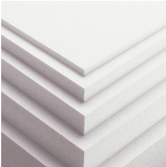
Figure 3. EPS used in constructions
