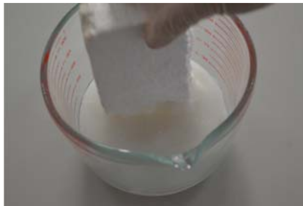
Figure 8. Polystyrene in propanone
