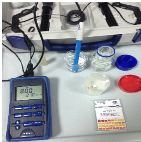
Figure 2. Determination of pH with pH sensor
