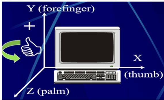
Figure 6. Spatial orthogonal 3D co-ordinate system XYZ (local)
