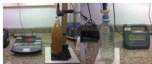
Figure 2. Rice husk water filtration system (Viana, 2016)
