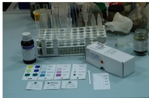
Figure 7. Hanna Instruments N, P, K analysis kit for soil sample analysis
