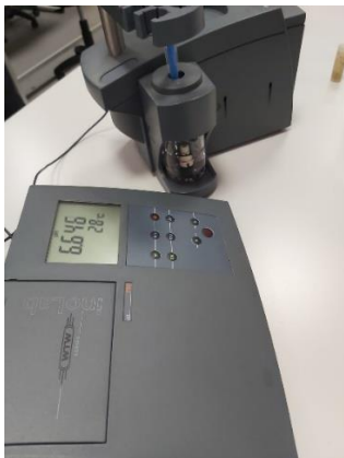
Figure 11. Results of electrochemical analysis of soil samples from the Nicula family household, 2020 - pH determined with WTW laboratory pH meter
