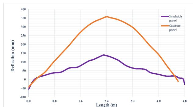
Figure 13. Deflection comparison between the two façade systems
