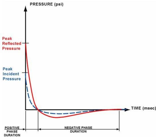
Figure 2. Air-blast as a function in time (FEMA 427)
