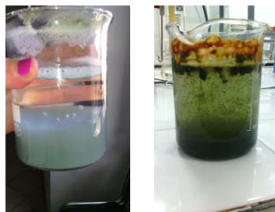
Figure 5. Sludge resulted from EC with iron electrodes (right) and aluminium electrodes (left).
