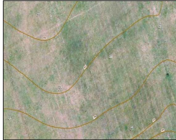
Figure 7. Contours with 1 meter equidistance
