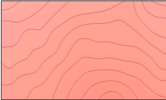
Figure 9. Contours based on SPLINE interpolation
