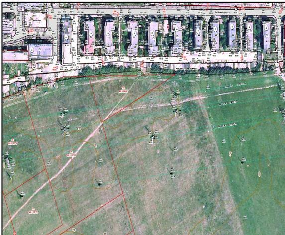
Figure 6. Sector of the topographic plan overlapped above the orthophoto map
