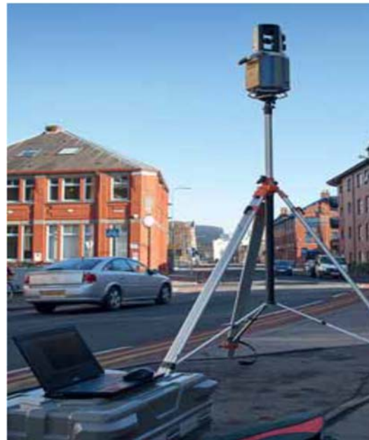
Figure 7. Laser scanning from an extra tall tripod
