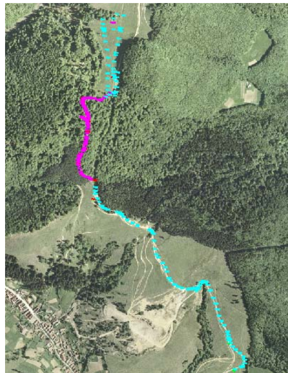
Figure 5. Points of detail taken over and RTK traverse
