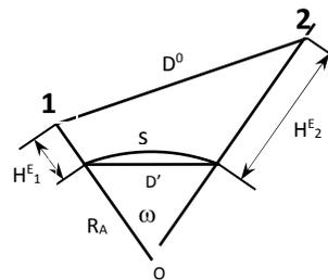
Figure 4. Reducing distances to reference surface
