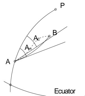
Figure 1- Reduction correction of the geodesic line
