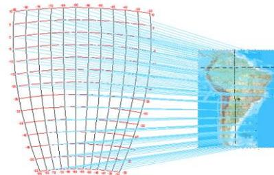
Figure 4-Georeferencing a scanned image
