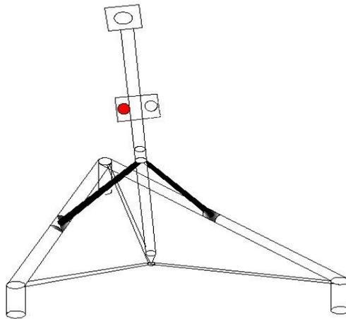
Figure 6. Incorrect position of prism
