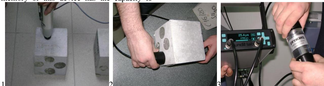
Figure 6. Images from the tests: 1. Digi Schmidt, 2. Pundit Lab, 3. Pundit Lab device calibration
