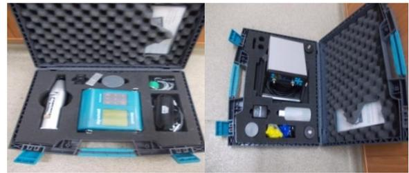
Figure 5. The equipment Digi Schmidt (left) and Pundit Lab (right)
