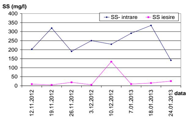
Figure 2. Evolution of concentrations of suspended solids leaving the SE entry
