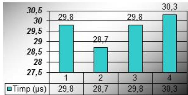
Figure 8. Determination of the propagation time of ultrasound
