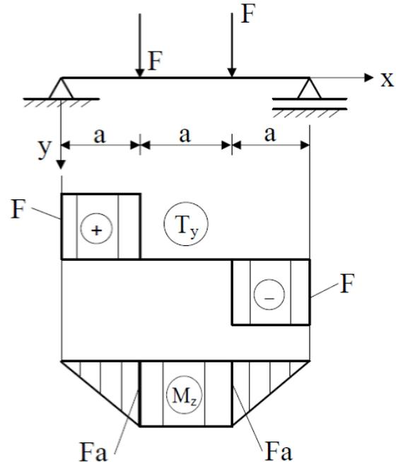
Figure 5. Bending test diagram
