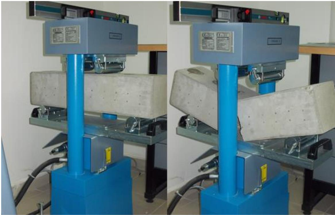
Figure 9. Bend testing on universal press SERVO PLUS Evolution
